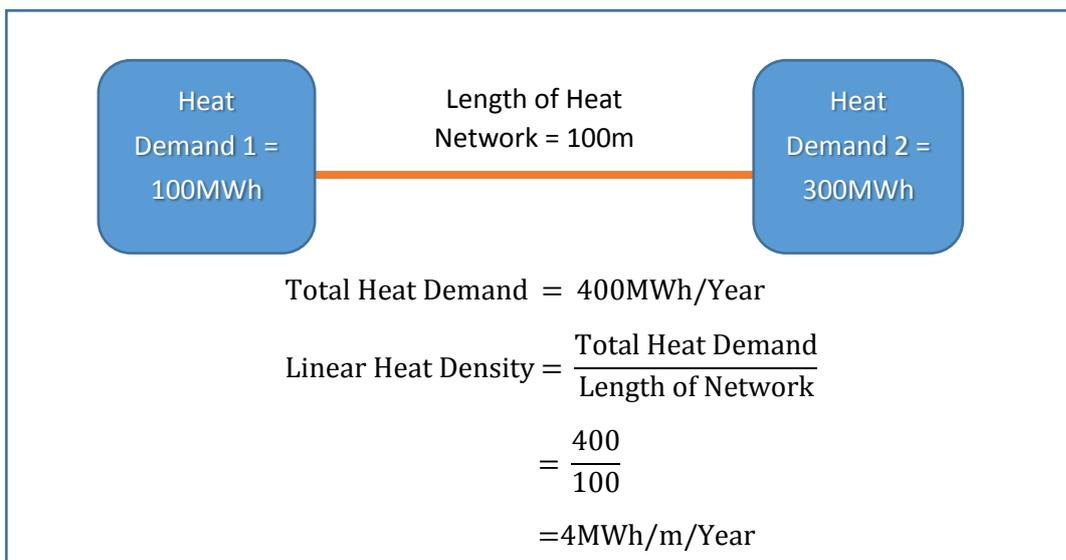
Figure 1 Calculation of linear heat density
